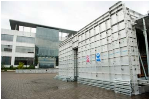
PreMold Aluminum Formwork
